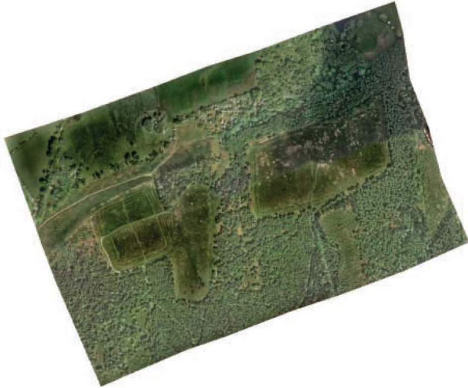
Figure 13. Digital orthophotograph of Roman Camps at Cawthorn, U.K. created from 15 vertical aerial photos (image: Bewley 2003, used with permission ©Wiley InterScience).
