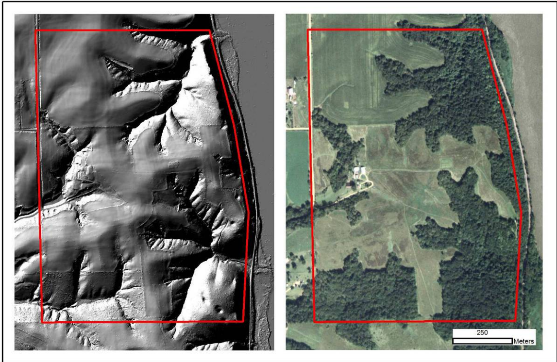
Figure 42. Clinton County test. AOI delimited in red. Left image is BE DEM shaded relief, right is 2008 NAIP true color imagery to show vegetation cover.
