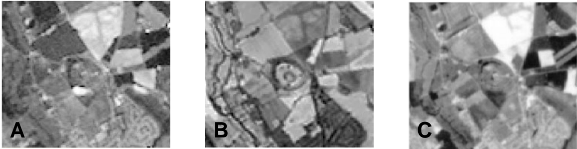
Figure 11. Comparison between Landsat TM Multispectral and SPOT panchromatic images. Center of each image is the Iron Age hillfort and later medieval site at Old Sarum, Wiltshire, U.K. A) Landsat TM visible bands 1-3, B) Landsat TM near-infrared band 4, C) SPOT panchromatic image (image adapted from Fowler 2002, used with permission ©Wiley InterScience).
